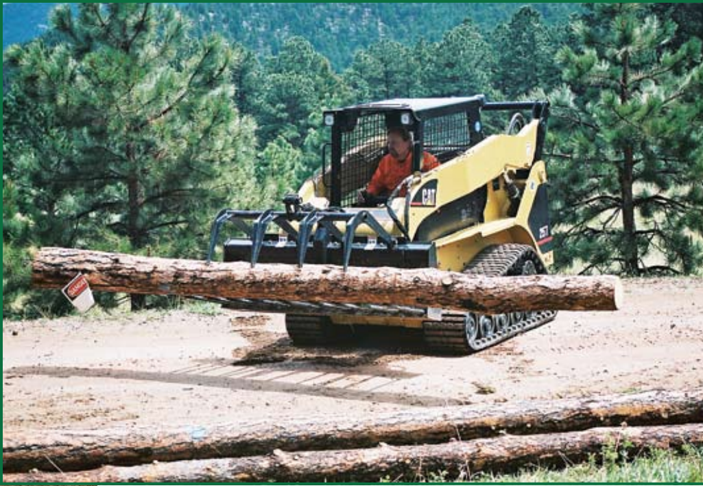
A skidsteer readies trees to be utilized as fencing at the Cal-Wood Education Center in Boulder County.
